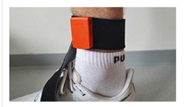
We investigate if amateur runners exhibit load asymmetries in their limbs and whether FFP2 masks may have an impact on then We use 5 smart inertial measurements units (Xsens MTw Awinda) attached to the tibiae, the sacrum and the scapulae to monito peak accelerations during each running cycle. We compare trails run under shoed and barefoot conditions as well with and with wearing FFP2 masks. Statistical analyses show some intriguing effects.
